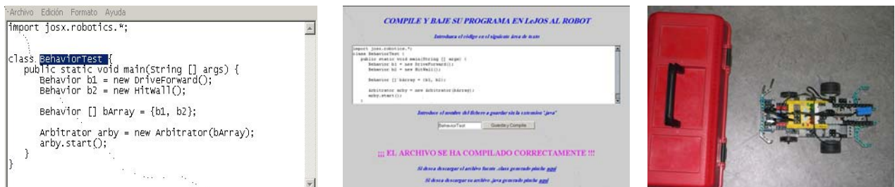
Figure 2. Example of use Editing the program BehaviorTest.java (left). Compilation and robot download (center). Visualization through the web cam (right).
